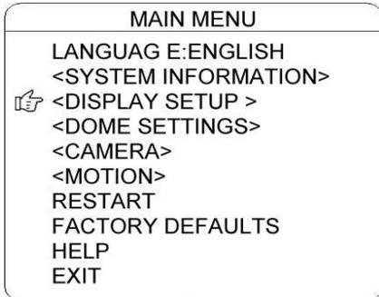
Display setup allows the user to define the way to display the dome titles on the monitor.
