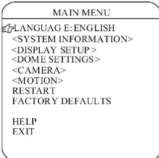
The user can check the dome system information as required. The system information includes: Dome ID, dome address, baud rate, protocol, temperature, voltage, alarm info, dome title, version, date, time, and temperature scale.
